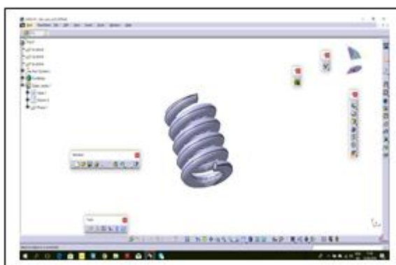
Figure 4. The CAD model of the circular cross sectional helical spring saved in stl format
