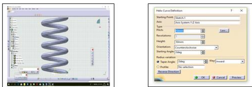
Figure 2. Left – Generating of 3D model; Right – Generating of helical springs in CATIA with option Helix Curve Definition
