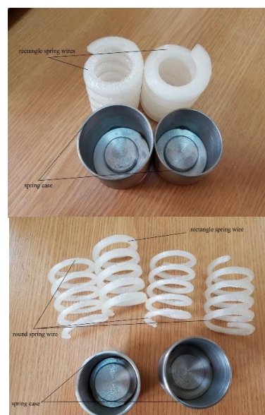
Figure 9. Rectangle and circular spring wires realized by FDM (Fused Deposition Modeling)
