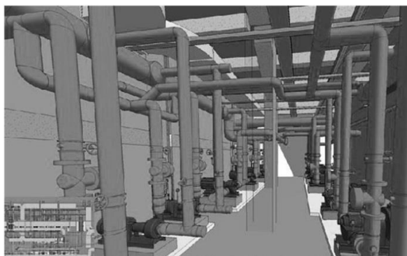
Figure 2: The internal roaming map of the three-dimensional model building
