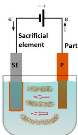
Figure 7: Flow of oxide particles from the part to the sacrificial element
