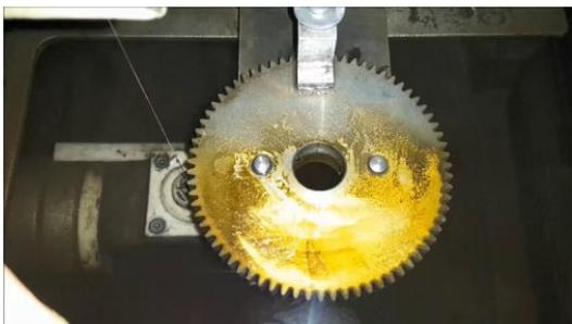
Fig. 5. Heavy oxide deposits on part and machine after the process
