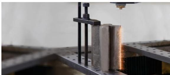
Figure 1: Electrical discharge machining on a metallic part
