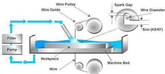
Figure 2: Wire EDM working principle
