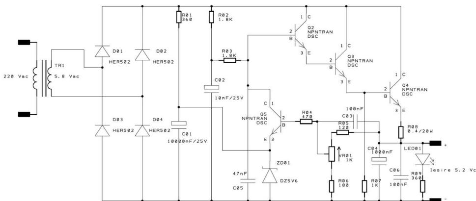
Fig. 6. Electrical diagram with the controllable DC power source
