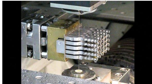
Figure 3: Wire electrical discharge machining
