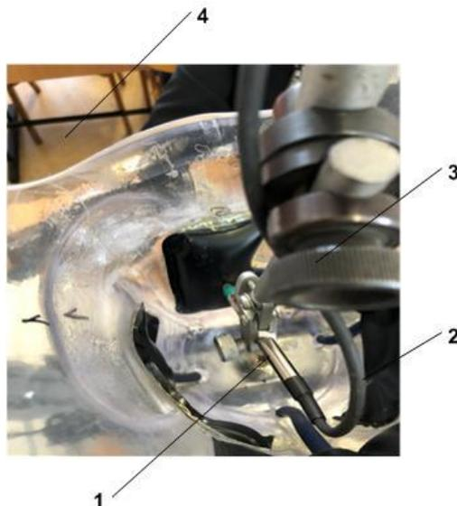
*Figure 5: The maximum level of deformation for the inflated cell*
