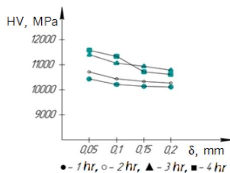
Figure 7: Effect of microhardness of cyanided at 550 °C
