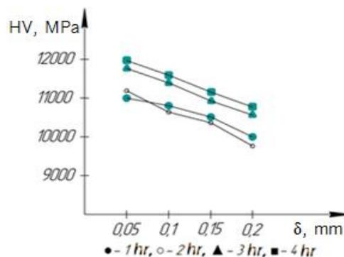
Figure 8: Effect of microhardness of cyanided at 620 °C
