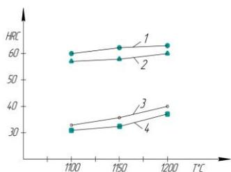
Figure 4: Tempering and quenching temperature effect on the hardness of P6M5. Tempering: 1 – 560 °C, 2 – 620 °C, 3 – 700 °C, and 4 – 730 °C
