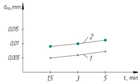
Figure 5: Effect of quenching time on the austenite grain size of P6M5 at 1200 °C. Tempering: 1 – 560 °C, 2 – 620 °C
