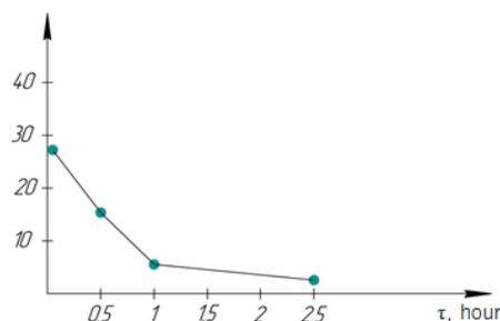
Figure 6: Effect of tempering at 560 °C on the amount of austenite of P6M5 quenched at 1200 - 1300 °C
