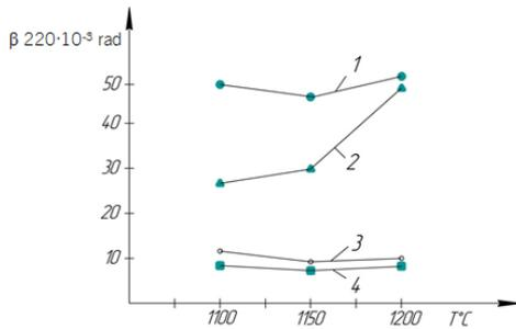
Figure 2: Tempering and quenching temperature affect the wideness of the physical line(β) of P6M5. Tempering: 1 – 560 °C, 2 – 620 °C, 3 – 700 °C, and 4 – 730 °C
