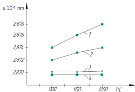
Figure 3: Tempering and quenching temperature effect on the parameters of crystals of P6M5. Tempering: 1 – 560 °C, 2 – 620 °C, 3 – 700 °C, and 4 – 730 °C
