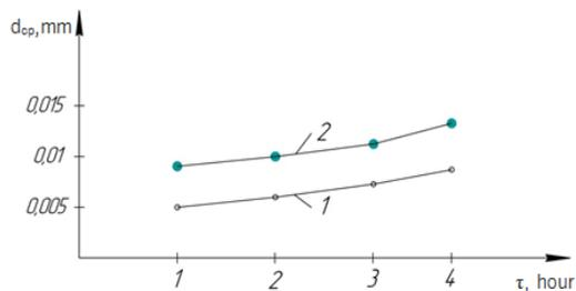
Figure 6. Effect of quenching time on the depth of the diffusion layer of P6M5. Tempering: 1 - 560 °C
