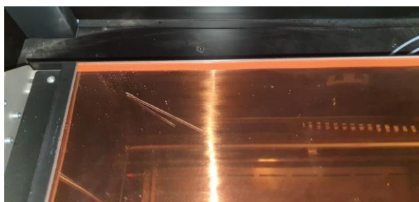
Figure 5: The extruder hits and scratches the print bed
