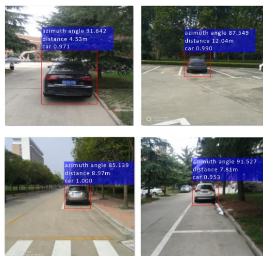
Figure. 9. Vehicle Location Test Results
