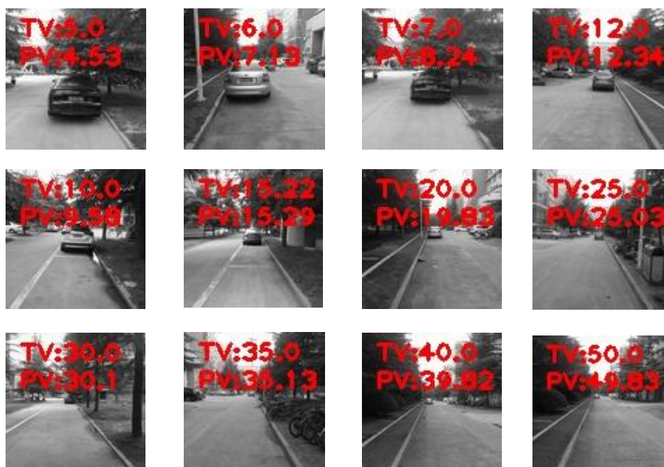
Figure 6. Distance detection results of preceding vehicle
