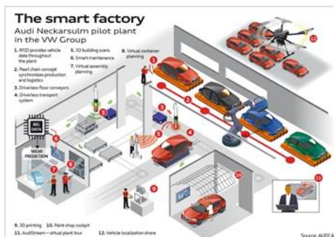
Figure 7: The smart factory - Audi Neckarsulm pilot plant in the VW Group [Source: AUDI AG]
