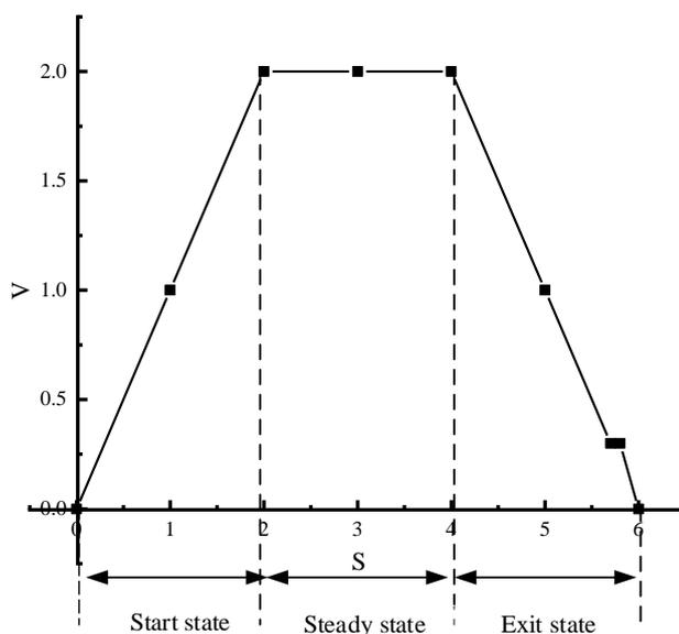
(a) The speed change of the manipulator in the process of the movement
