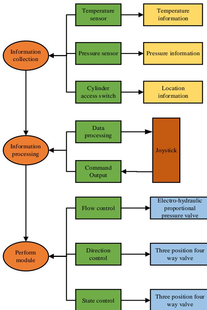
Figure 2: The overall design scheme of the control system of the manipulator
