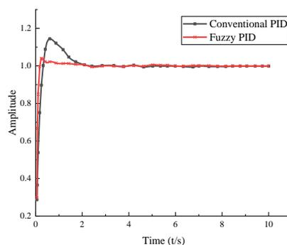
(a) Comparison of fuzzy PID and conventional PID without interference of external load
