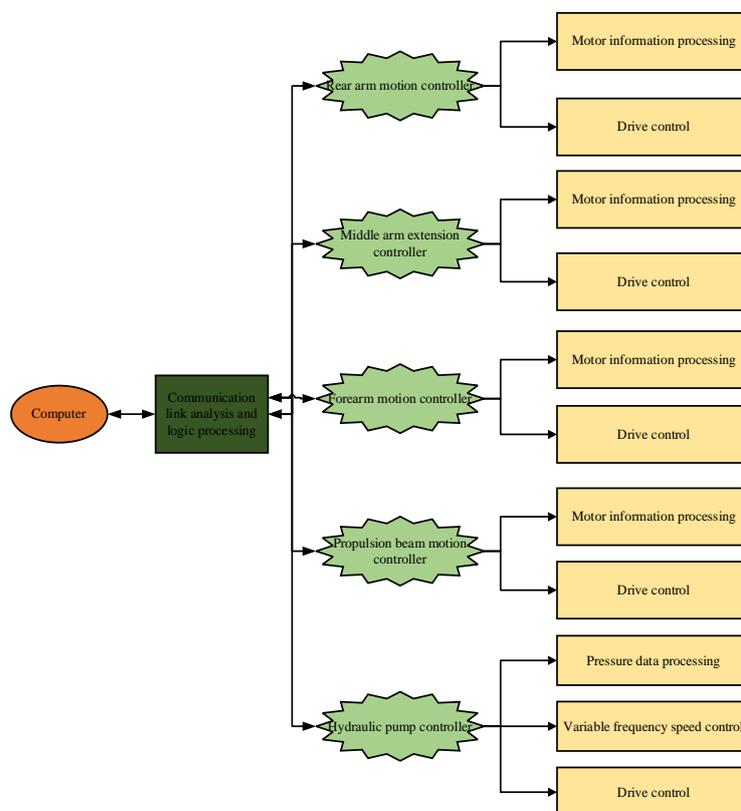
(b) The diagram of the overall design of software system of the electronic drive control system of the hydraulic joints of the manipulator
