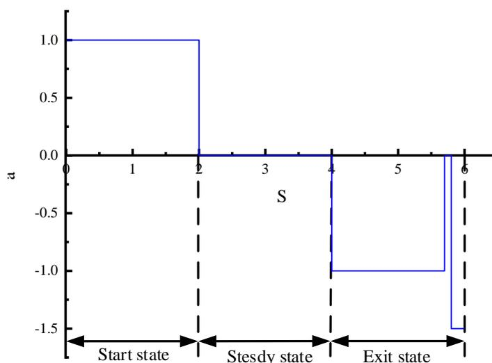
(b) The acceleration change of the manipulator in the process of the movement
