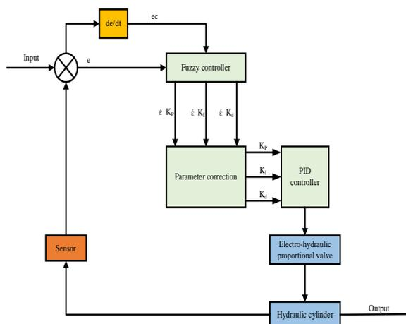
(b) The structure of the fuzzy PID controller
