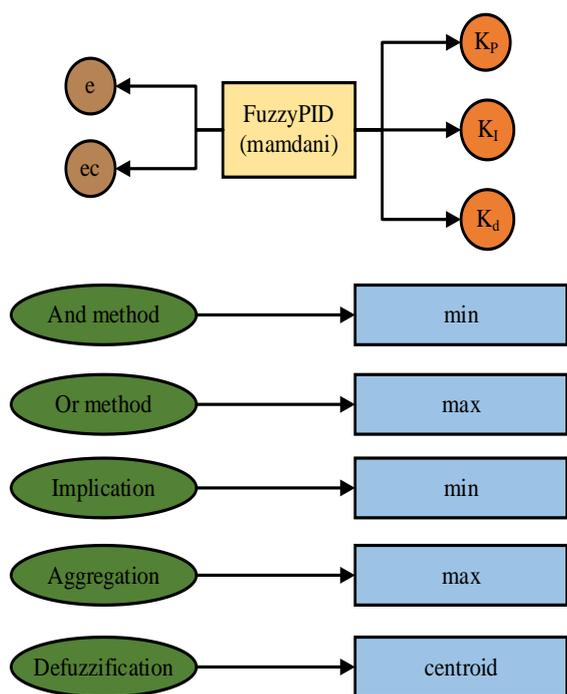
Figure 7: The setting of fuzzy inference system and fuzzy logic algorithm
