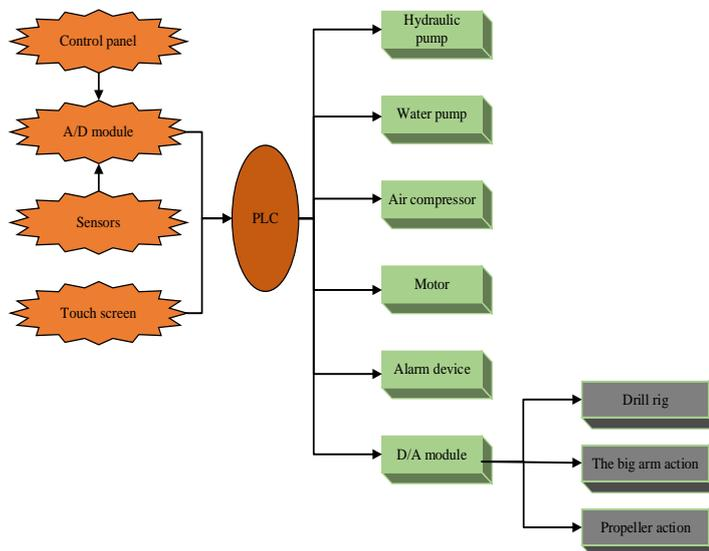
(a) The diagram of the overall design of hardware system of the electronic drive control system of the hydraulic joints of the manipulator
