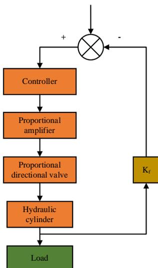
Figure 4: The hydraulic electronic drive control system of the manipulator
