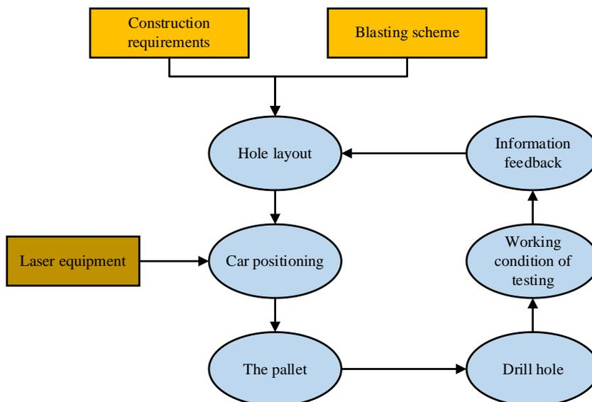
Figure 1: The main work process of the jumbo
