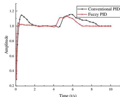
(b) Comparison of fuzzy PID and conventional PID when impacted by 10000N external load
