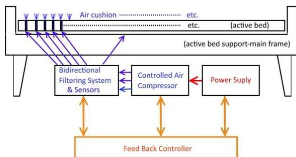
Figure 2 - General diagram of the Testing Stand
