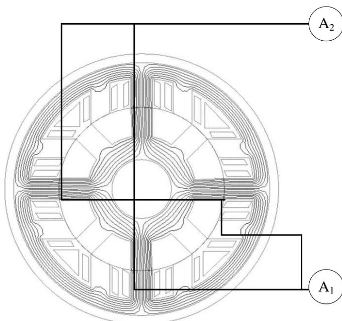
Figure 1: Structure of the three-phase doubly salient reluctance motor
