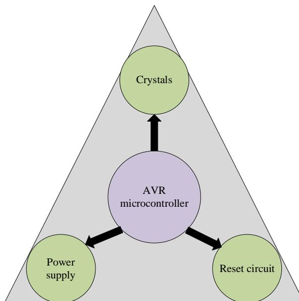
Figure 3: Elements of the minimum system of SCM
