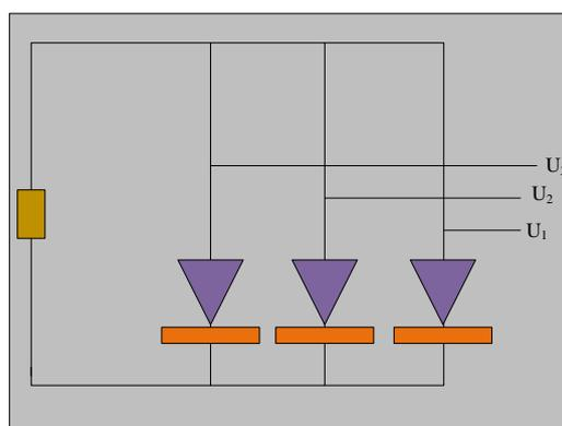
Figure 2: Structure of the three-phase full-wave rectifier circuit
