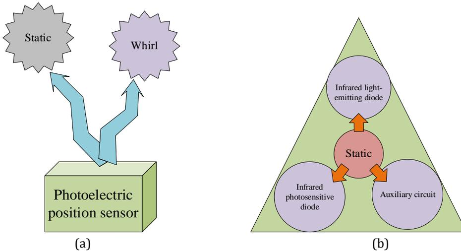
Figure 5: Composition of the photoelectric position sensor (a) Elements of the macroscopic composition, (b) Static elements of the macroscopic composition)
