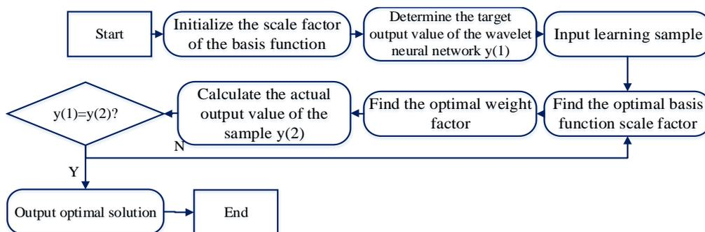
Figure 2: Flowchart of fault diagnosis
