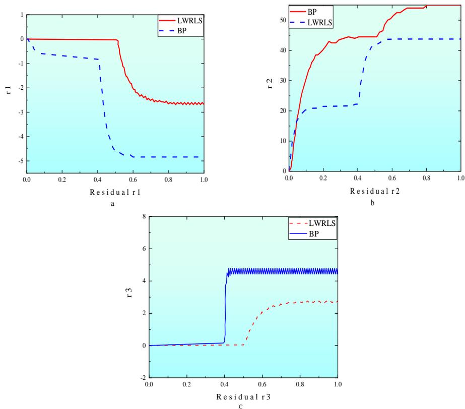
Figure 9: Residual waveforms of open-circuit faults under the two algorithms (a: waveform of residual r1; b: waveform of residual r2; c: waveform of residual r3)
