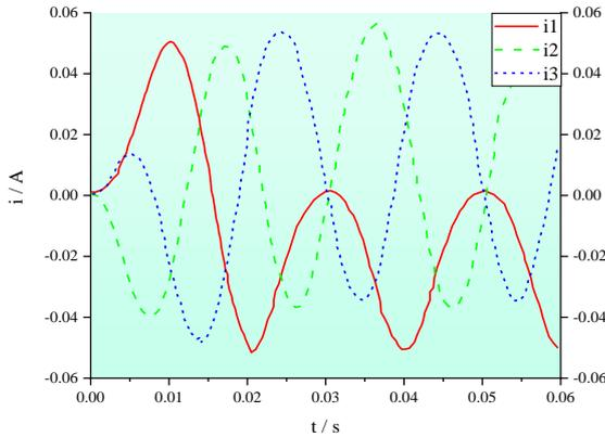
Figure 6: Waveform of inverter's three-phase current output during open circuit fault
