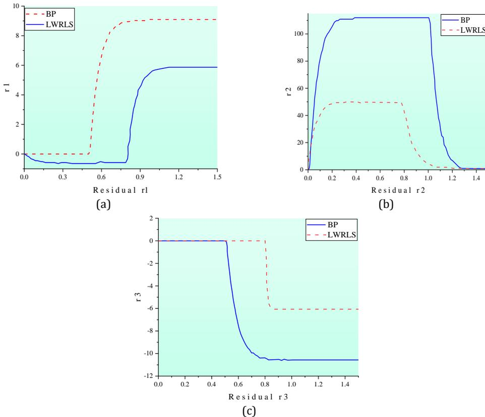
Figure 8: Residual waveforms of short-circuit faults under the two algorithms (a: waveform of residual  $r_1$ ; b: waveform of residual  $r_2$ ; c: waveform of residual  $r_3$ )
