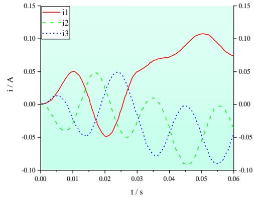
Figure 7: The three-phase current output waveform of the inverter during short-circuit fault
