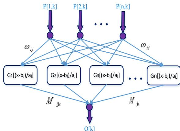
Figure 1: Model structure of WNN
