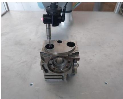
Figure 2: Touch probe measurement method
