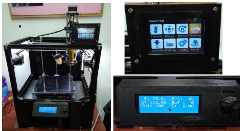
Figure 4. 3D printer prototype used in the food industry: a-general view; b – electronic control panels
