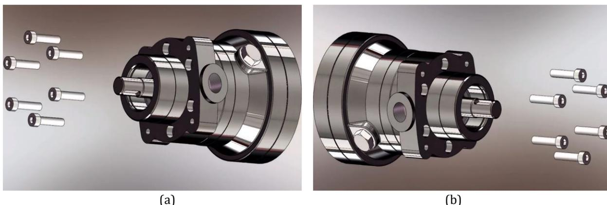
Figure 4: The simulation diagram of the specific disassembly situation of the first step (a: disassemble the long hexagon screw 1; b: disassemble the long hexagon screw 2)
