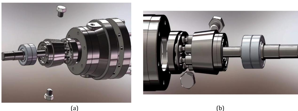
Figure 6: The simulation diagram of the disassembly of components in the third step (a: disassemble the front and rear oil distribution plate; b: disassemble the middle pump body, front and rear cylinder block and piston components)
