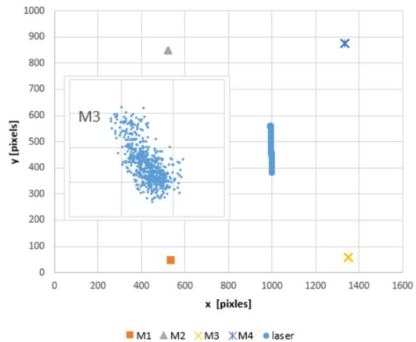
Figure 26: Detected markers positions and LASER trace. Zoomed in, the scatter of marker M3 position
