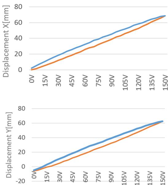
Figure 13: Characterization of the static behavior of piezoelectric actuators, variant with the adhesion of the mirror on the surface. Displacement in mm, at a distance  $d = 0.80m$ .
