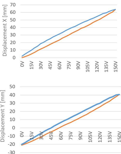
Figure 12: Characterization of the static behavior of piezoelectric actuators, version with 3D support. Displacement in mm, at a distance  $d = 0.77m$ .
