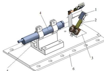
Figure 6: Stand for testing bimorph actuators and bidirectional LASER beam guidance system mechanical structure: 1-mirror; 2-piezoelectric bimorph actuator; 3-hardening support; 4-fiber optic LASER; 5- LASER support; 6- base plate.
