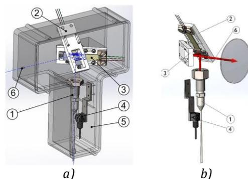
Figure 4: Constructive solution for vibration compensation system with two orthogonal LASER deflection systems, in two directions [13].
