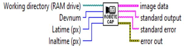
Figure 15: Input – output wiring of the “RobotEyez.vi”
