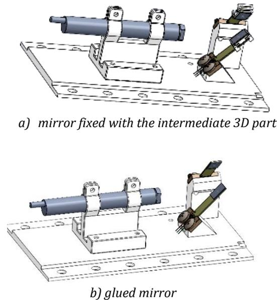
Figure 10: The constructive solution of the tremor compensation system in two variants.
