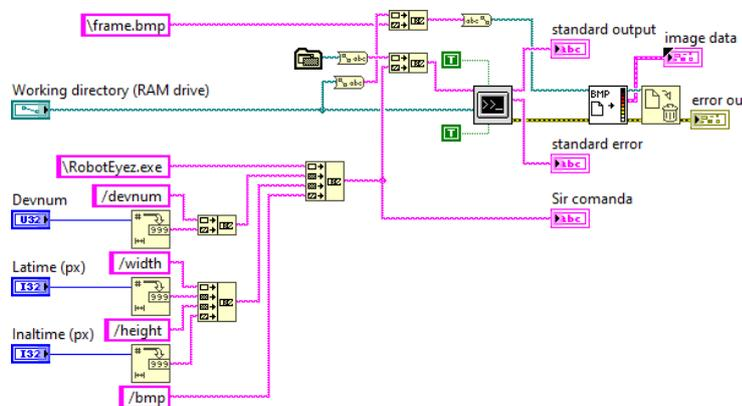
Figure 16: “RobotEyez.vi” code
