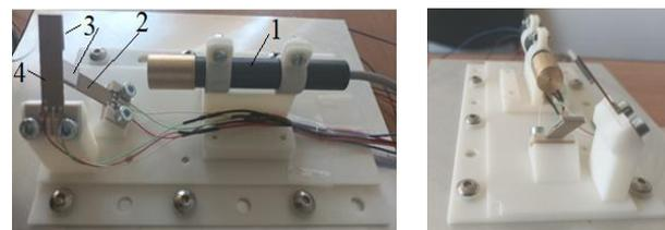
Figure 11: Stand for characterizing the static and dynamic behavior of piezoelectric actuators and the bidirectional laser beam guidance system. Two-way LASER deflection system 1-LASER; 2,4-actuators; 3-mirrors.
