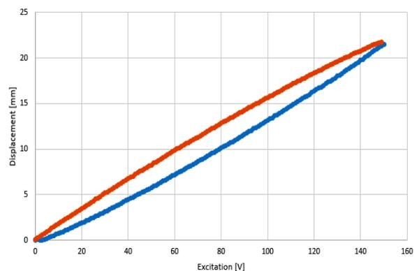
Figure 27: Measured hysteresis curve for the piezo actuator type PB4VB2W
