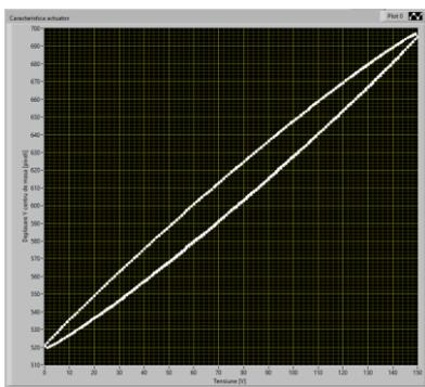
Figure 24: Vertical actuator characteristic drawn as pixel position vs. supply voltage
