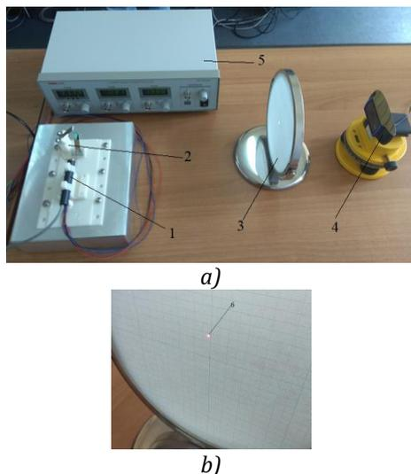
Figure 9: Stand for testing bimorph actuators and bidirectional LASER (piezo deflection system) guidance system. a) overview and b) spot details: 1-LASER; 2-deflection system with piezoelectric actuators; 3-gratulated translucent screen; 4-webcam; 5-voltage generator for piezoelectric actuators; 6-spot laser lights.
