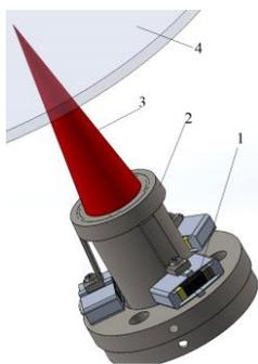
Figure 1: Stewart platform amplification system assembly: 1-piezoelectric actuator with displacement amplification; 2-mechanical system with compliant mechanism; 3 - LASER beam; 4 - work surface.
