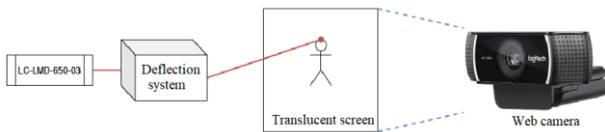
Figure 8: Schematic diagram of the stand for characterizing the bidirectional LASER beam guidance system.
