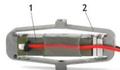
Figure 2: Piezoelectric microactuator: 1- Stack piezoceramic pills; 2- metal frame [12].
