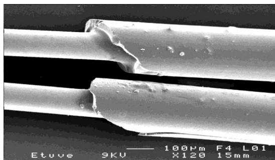
Figure 3: Stripped fibers
