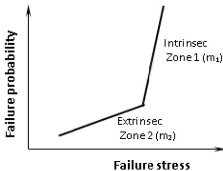
Figure 4: Failure stress bimodal distribution
