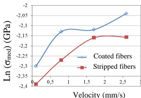
Figure 10: Median strength for coated and stripped fibers under inert atmosphere versus faceplate velocity
