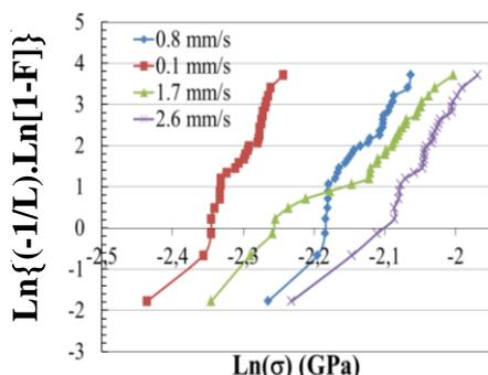
Figure 8: Weibull curves for coated fibers in inert atmosphere
