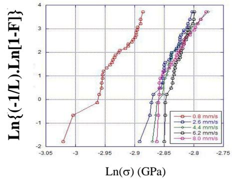
Figure 5: Weibull curves for coated fibers in the air
