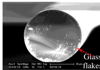
Figure 11: Cross area of stripped fiber after failure
