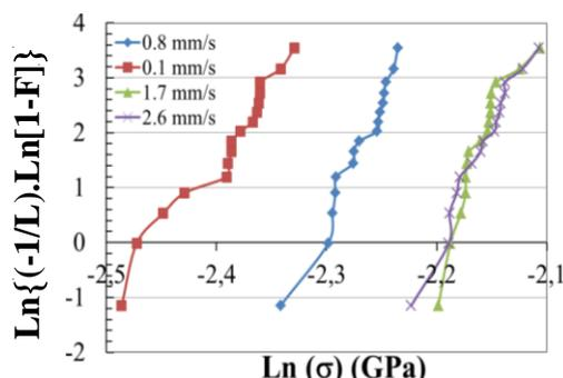
Figure 9: Weibull curves for stripped fibers in inert atmosphere
