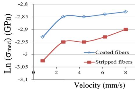
Figure 7: Median strength for coated and stripped fibers in the air versus faceplate velocity
