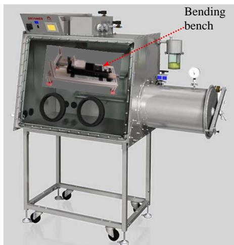
Figure 2: Compact glove box with purification system (Jacomex GP Campus T2)
