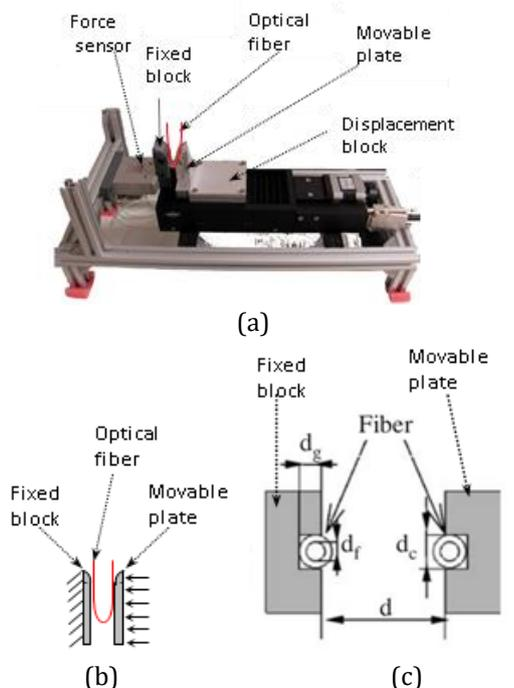
Figure 1: (a) Bending bench used; (b) and (c) fiber between thrust blocks
