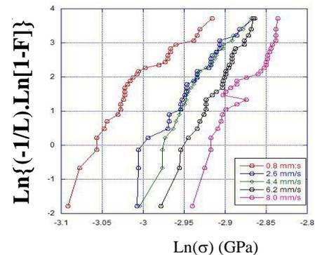
Figure 6: Weibull curves for stripped fibers in the air
