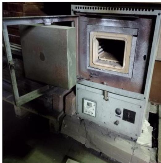
Figure 2: Muffle furnace brand SNOL-1,6,2,5.1/11-I2M
