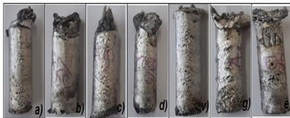
Figure 6: Castings. a-aluminum alloy grade A-8176; b- 5 gr wrapped LiF added sample; c- 10 gr wrapped LiF added sample; d- 15 gr wrapped LiF added sample; v-5 gr not wrapped LiF added sample; g-10 5 gr not wrapped LiF added sample;
