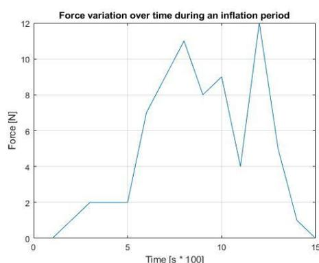
Figure 5: The pressure force variation on time during the inflation period.
