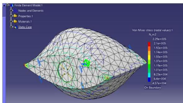
*Figure 2: The FEM analysis of the thin wall cell.*
