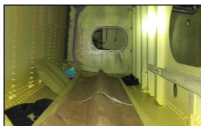
Figure 19: Removal of traces of kerosene left in the central fuel tank of the Boeing 737-300 aircraft
