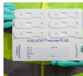
Step 2 – After 15 min examine the result Figure 5. Fuelstat resinae plus - fuel test kit [23]
