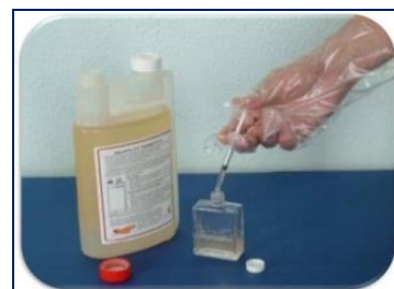
Step 1 –With the help of an syringe add 0,5 ml fuel to the Microbmonitor2 bottle. Close the bottle and put a label
