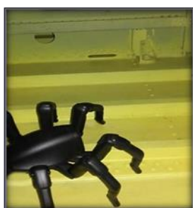
Figure 21: The hexapod mobile robot inside the central fuel tank of the Boeing 737-300 aircraft
