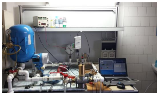
Figure 2: Specialized equipment for calibration in-line
