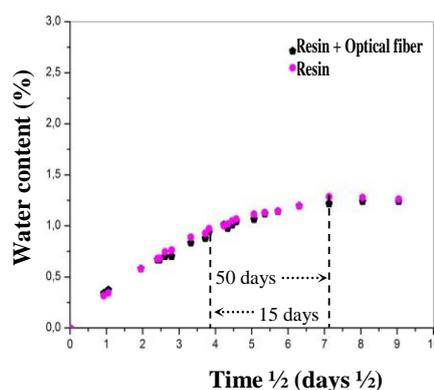
Figure 4: Water content versus immersion time for vinylester resin samples
