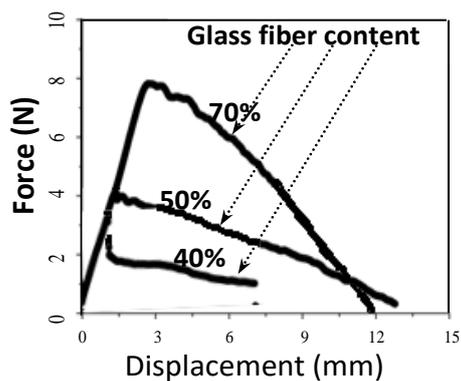
Figure 8: Force-displacement curves from pull-out test for composite samples aged in water for 60 days
