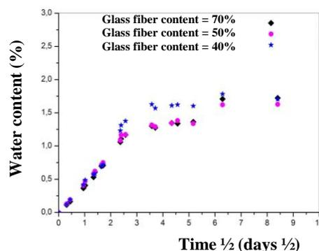
Figure 5: Water content for different glass fiber volume content for composite with-vinylester resin
