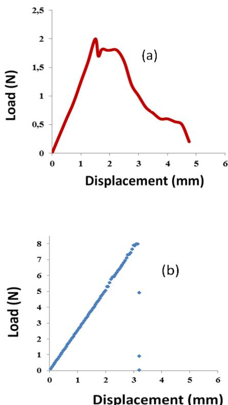
Figure 3: Force-displacement curves of the unaged O.F./Polyester (a) and O.F./Vinylester (b) samples obtained owing to pull-out tests.
