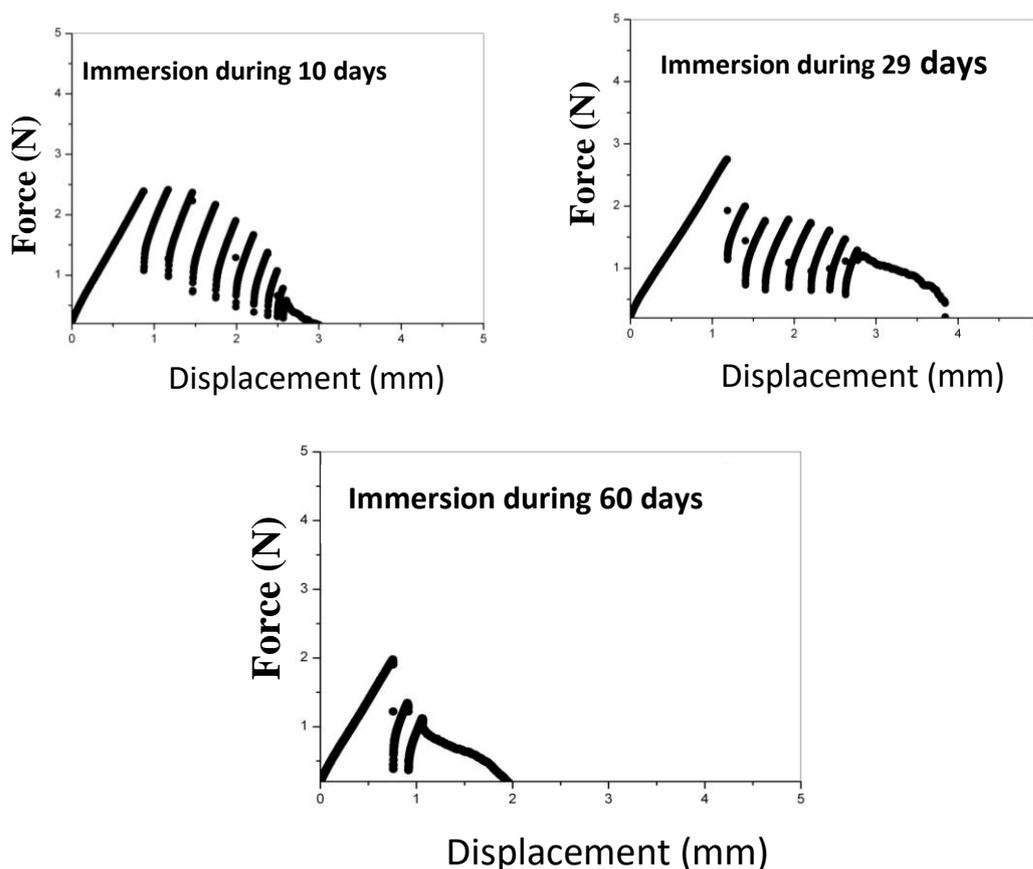
Figure 7: Force-displacement curves for different immersion durations in water for optical fiber embedded in vinylester resin samples and submitted to pull out test.
