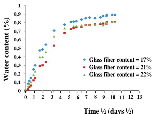
Figure 6: Water content for different glass fiber volume content for composite with polyester resin
