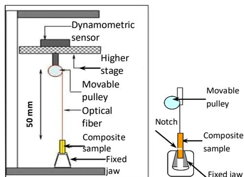
Figure 1: Description of the dynamic tensile test bench and detail of used composite sample
