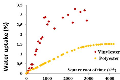
Figure 2: Moisture absorption curves for two resin samples
