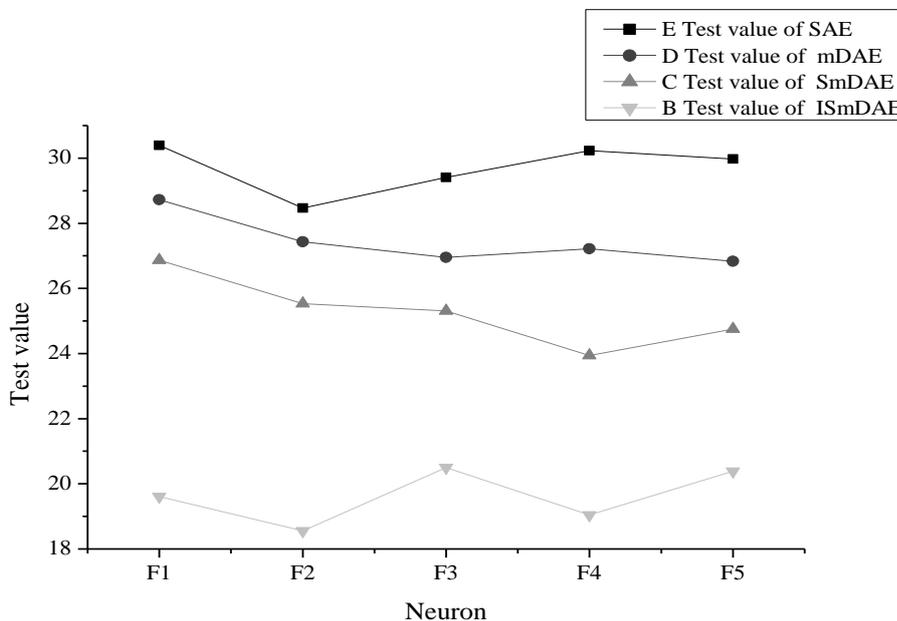
Figure 7: Comparison of test results of various encoders under the electronic circuit fault data of the three-spot resistance welder
