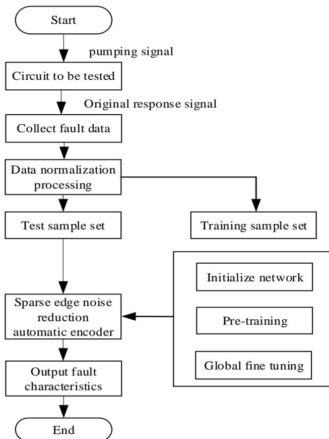
Figure 4: Feature extraction process of electronic circuit fault information of three-spot resistance welder
