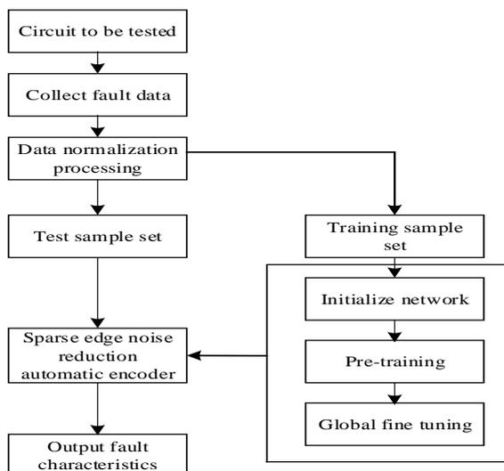
Figure 2. Mechanical fault extraction process of ISm DAE
