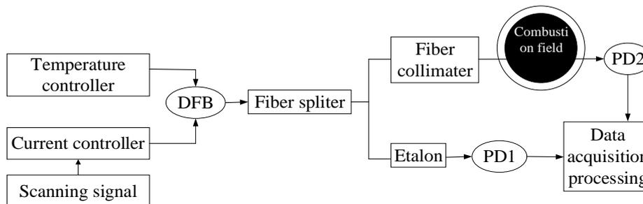
Figure 4. Two-dimensional reconstruction system of flat flame furnace temperature measurement based on TDLAS technology
