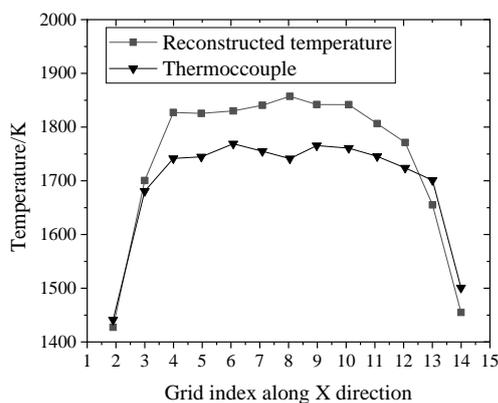
Figure 8: Comparison of thermocouple measurements and reconstruction results at several points along the X direction
