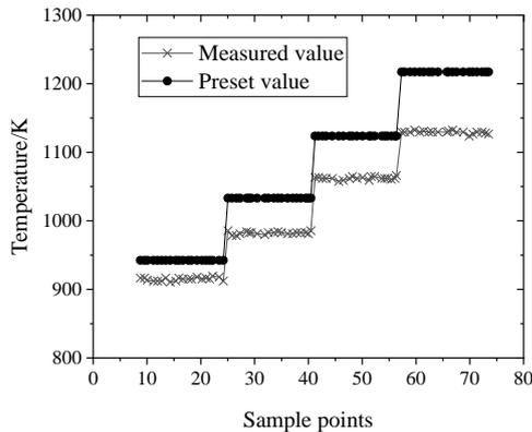
Figure 5. Comparison of temperature measurement results and setting results of high temperature tubular furnace
