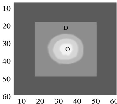
Figure 7: Temperature distribution of thermocouple measurement results
