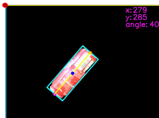
Figure 2.2.12 – Centroid coordinates and orientation
