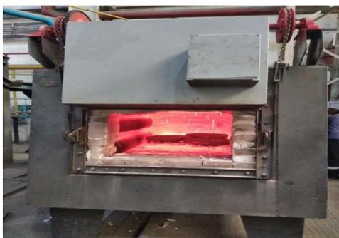
Figure 6: SNOL - 7.2 / 1100 muffle furnace for heat treatment of samples
