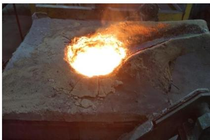
*Figure 3: IST is a high chromium cast iron liquefaction process in a 0.4 induction furnace*
