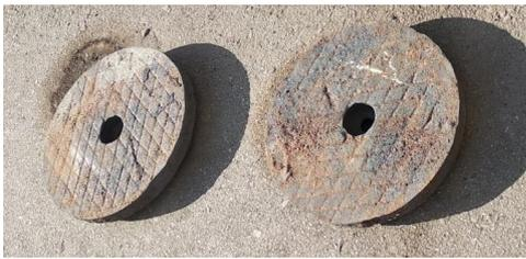
Figure 4: Appearance of disc cast in sand-clay mold
