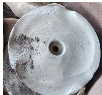
*Figure 2: A view of a disc cast that has become unusable*
