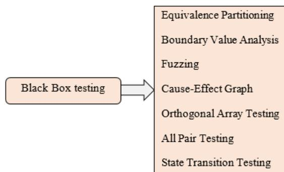
Figure 4. Types of testing Black box testing [9]
