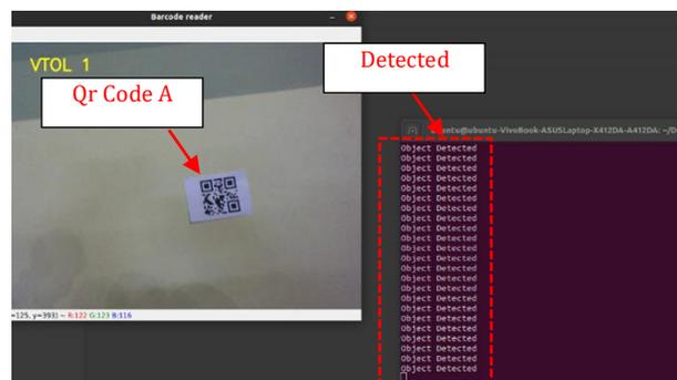
Figure 7 Monitor display of detection results on Qr Code A
