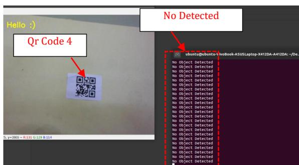
Figure 10 Display results monitor detection results on Qr Code D
