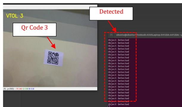
Figure 9 Display results monitor detection results on Qr Code C
