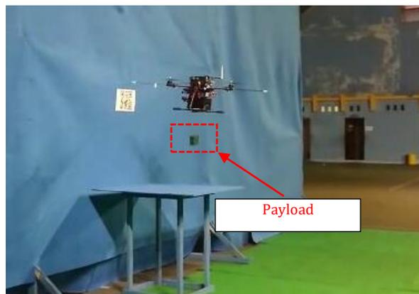
Figure 13. The quadcopter drops the payload
