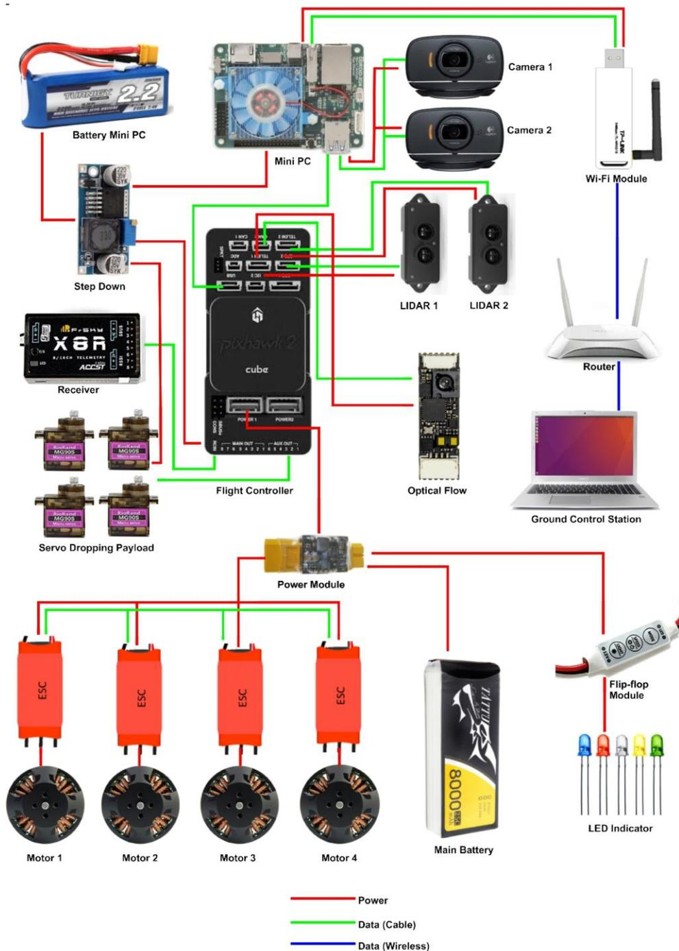
Figure 1. The quadcopter electronics circuit
