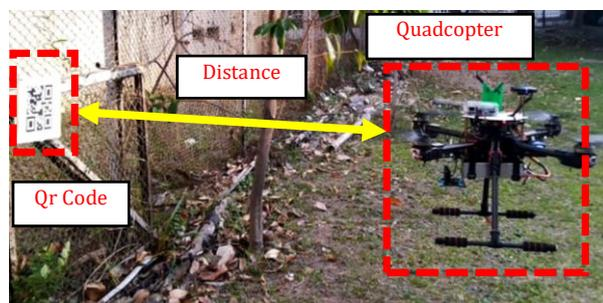
Figure 6 Functionality test data retrieval scheme
