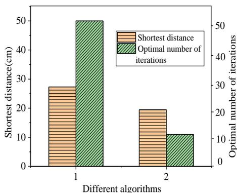
Figure 8: Comparison of parameters between common ant colony algorithm and improved ant colony algorithm under U-shaped obstacle terrain (1: common ant colony algorithm 2: improved ant colony algorithm)
