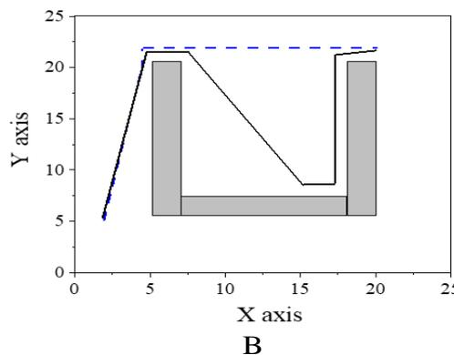
Figure 6: Path planning of robot in random terrain and U-shaped obstacle terrain (A: random terrain, B: U-shaped obstacle terrain (solid line represents common ant colony algorithm, and dotted line represents improved ant colony algorithm))
