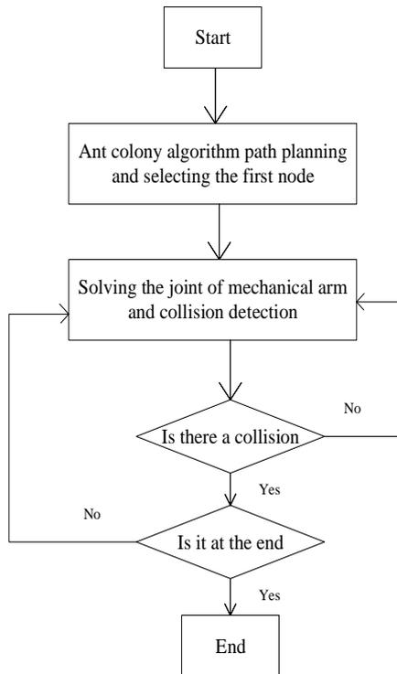
Figure 2: The flow chart of path planning of the mechanical arm under the condition of improved ant colony algorithm
