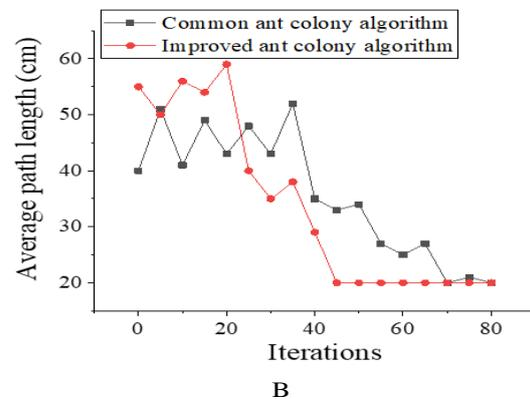
Figure 3: Comparison of convergence curve between improved ant colony algorithm and common ant colony algorithm (A: the change of path length with the number of iterations; B: the change of average path length with the number of iterations)
