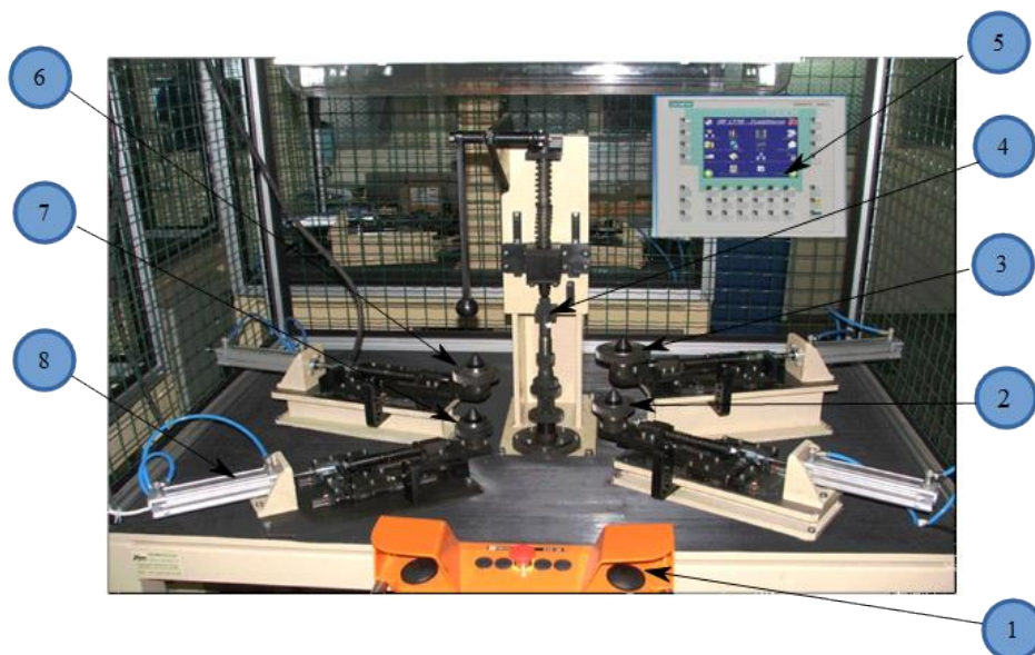
Figure 14: A unit used for checking gears II-V, determining side clearance (phosphate layer thickness), eccentricity and shocks, developed for DACIA RENAULT
