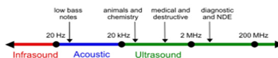
Figure 1: The Representation of sound vibrations depending on frequency and fields of application
