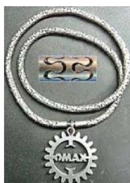
b) Chain made of a solid titanium tube (outer diameter is 0.64 mm)
