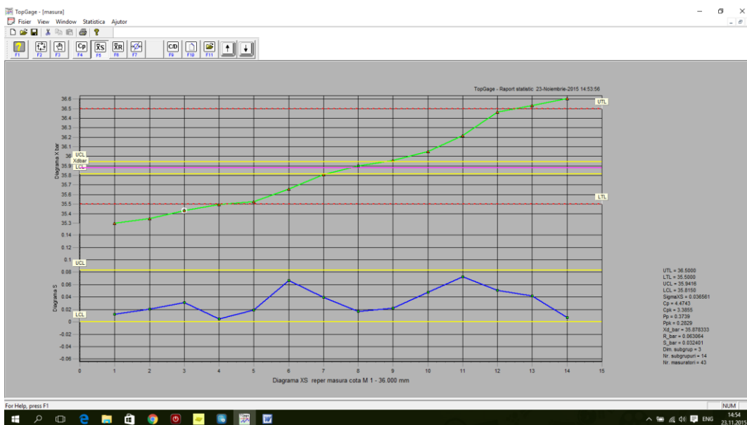
Fig.15 X-S chart – for bearing ring with nominal value of outer diameter 36 mm
