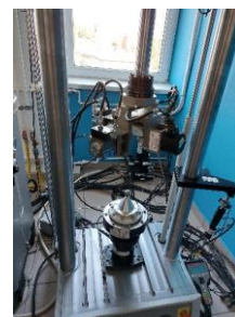
Figure 3: MTS Bionix Implants and Prosthetic Components Testing Equipment
