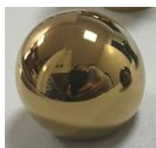
1.5 \mu\text{m} thick TiN thin film deposited by DC sputtering (a)
