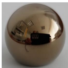
1.5 \mu\text{m} thick CrN thin film deposited by DC sputtering (c)
