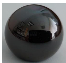
1.5 \mu\text{m} thick TiO 2 thin film deposited by DC sputtering (b)
