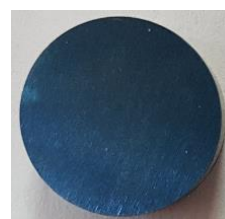
0.5 μm TiO 2 thin film deposited on CoCr substrate by DC sputtering
