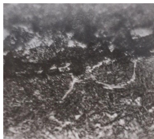
Figure 8: \epsilon - phase along the grain boundaries in the cyanated layer, x500
