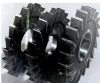
Figure 5: Cast bimetallic disk three-sided machining tools (diameter D=100 mm, B=6, 14, 12 mm)
