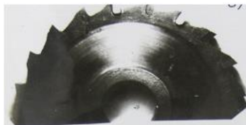
Figure 9: Cast bimetallic multi-blade tool: grooved milling tool
