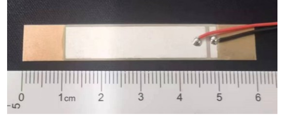
Figure 2: The rectangular piezoelectric beams as research objects
