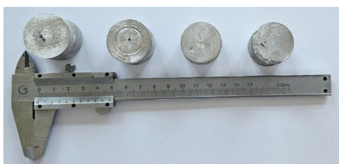
Figure 3: Samples cut to measure hardness.
