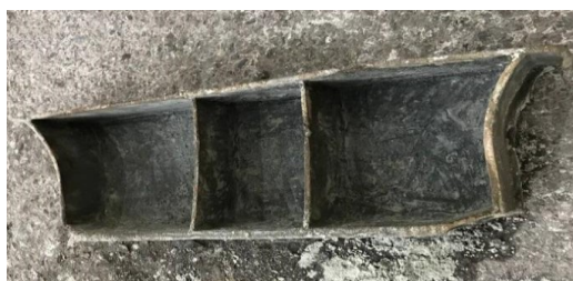
Figure 16: Detail of a thin-walled high-rise construction raised roof cast in gray cast iron in sand-clay moulds.
