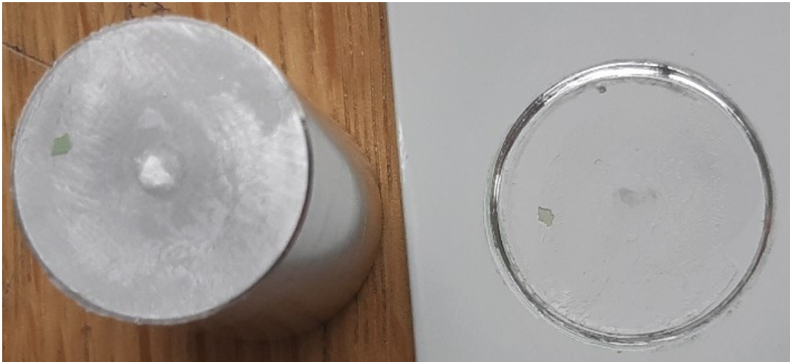
Figure 4: How the sample breaks when using Loctite Super Bond Universal adhesive
