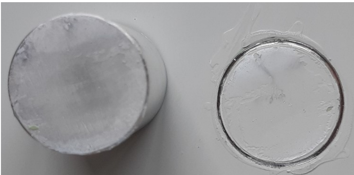
Figure 3: How the sample breaks when using Loctite Super bond Power Flex adhesive
