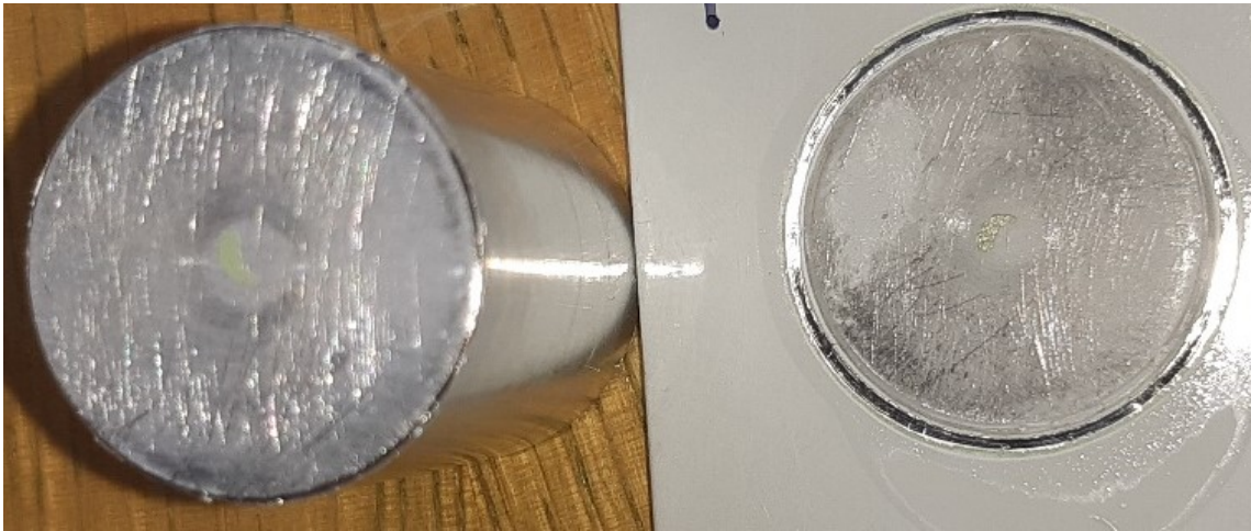
Figure 1: How the sample breaks when using Bison Super Glue adhesive
