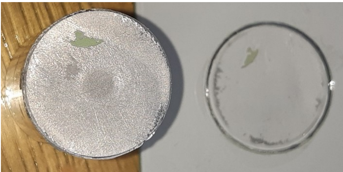
Figure 2: How the sample breaks when using Bostik Glue Fix adhesive
