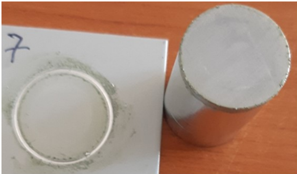
Figure 7: How the sample breaks when using Loctite 638 adhesive
