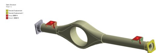
Figure 3: Load and constraint under full load statics
