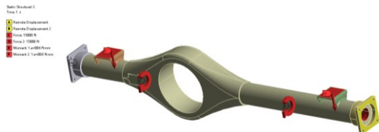
Figure 6: Load and constraints under maximum traction condition
