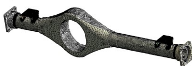
Figure 2: Mesh model of drive axle
