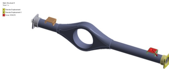
Figure 12: Constraint and load under the biggest lateral force
