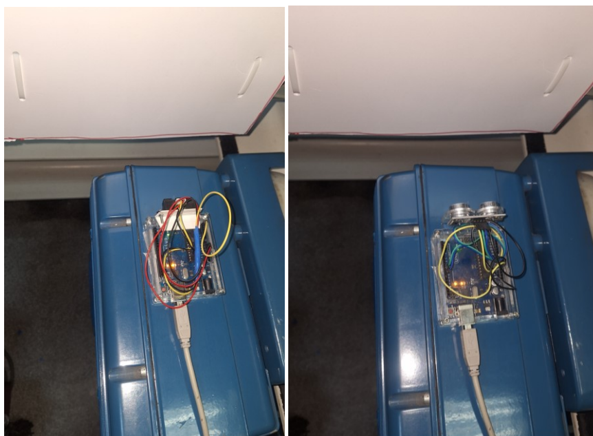
Figure 4: SM monitoring system - left with IR sensor and right with ultrasonic sensor
