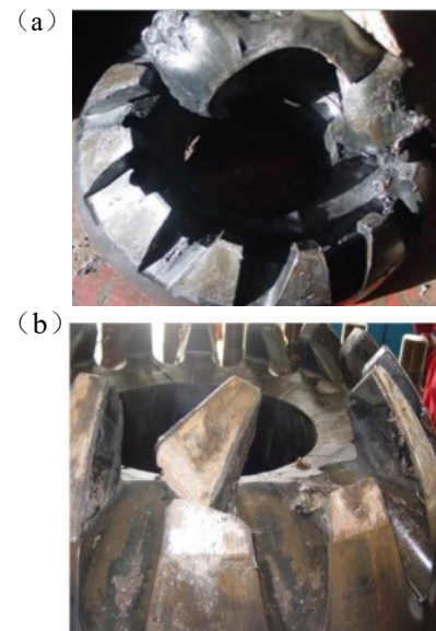
Figure 2: Failure photos of rubber core and support rib: (a) rubber core, and (b) support rib.
