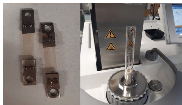
Figure 2: TMA sample on the left, sample inserted in the TMA device on the right.
