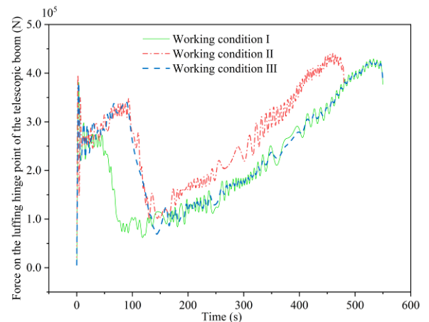
Figure 10: The force on the tail hinge point of the telescopic boom under different working conditions
