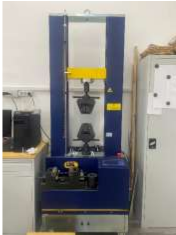
Figure 10: LBG TC100 Material Testing Machine
