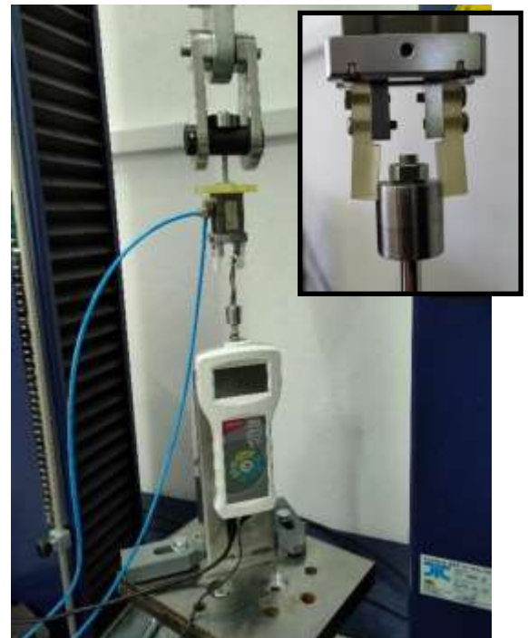
Figure 12: The experimental setup and the specimen between the jaws (in case of parallel gripper)
