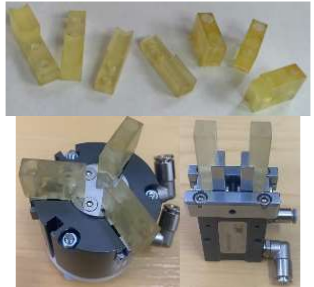
Figure 8: Resin jaws printed on the 3D printer Objet Eden 350V and attached to the grippers
