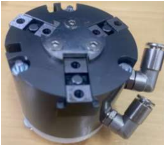
Figure 3: Pneumatic grippers with 3 jaws
