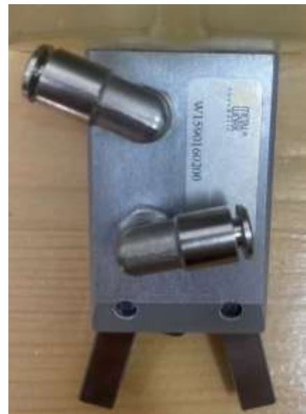
Figure 2: Angular pneumatic gripper
