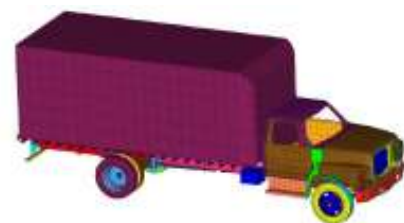
Figure 1: Vehicle finite element model of Ford F800
