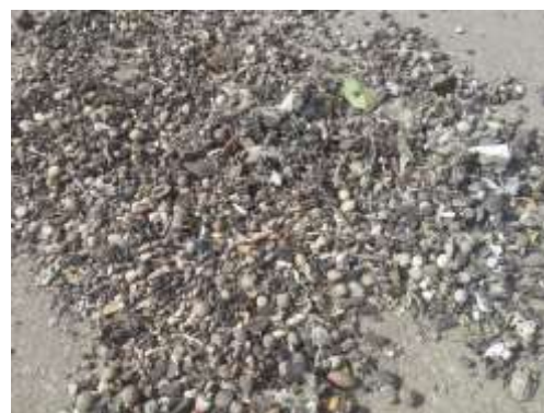
Figure 4: Large particles in the thickened product of the hydrocyclone
