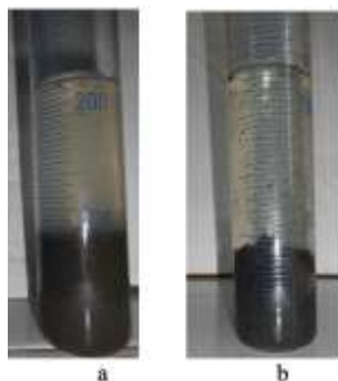
Figure 5: Samples of liquid waste after additional physicochemical treatment with model suspension and flocculant: a – excess activated sludge mixed with model suspension in a 3:1 ratio; b – centrifuge filtrate mixed with model suspension in a 1:1 ratio
