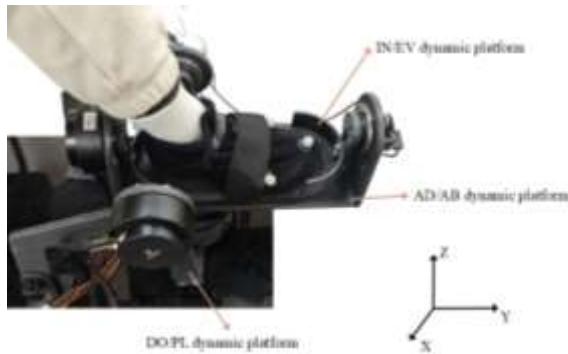
Figure 4: Ankle joint movement experimental device
