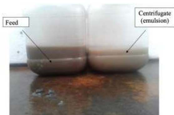
Figure 5: Photographs of the centrifuge feed and centrifugate
