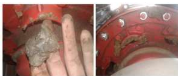
Figure 6: Photographs of fat deposits in the centrifugate discharge ports
