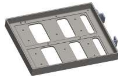
Figure 2: Structure diagram of the battery tray and lifting lugs
